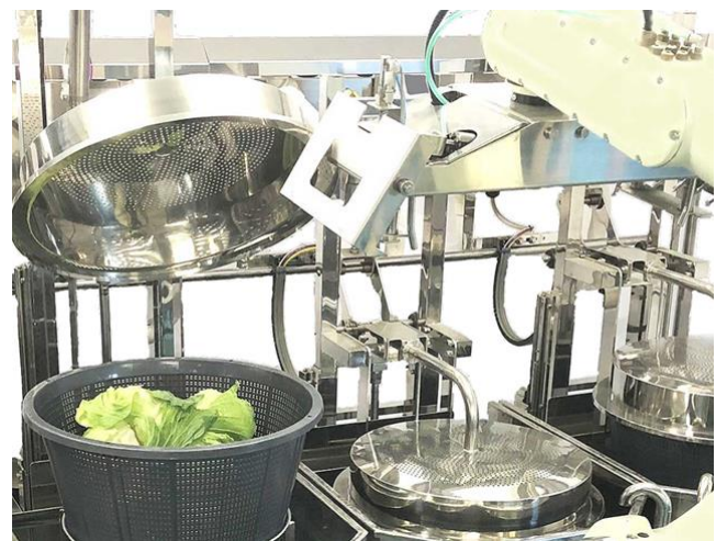
Fully automated washing/disinfection line
